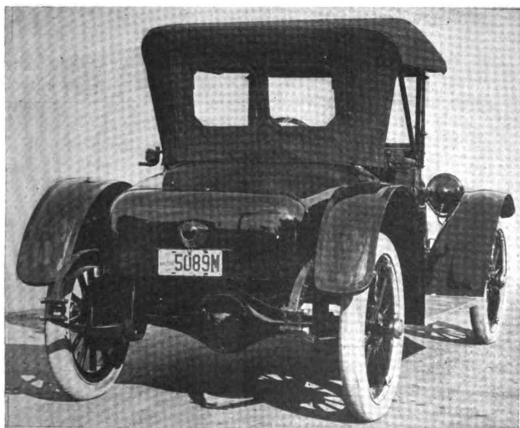
Left—Rear view of new Hupmobile roadster, showing tail light and license bracket mounted in the center. Right—Dash view, showing instrument board. Left—Lighting switch; center, speedometer; right, starting and ignition switch. All switches are controlled by Yale lock. Note pads on pedals
